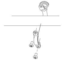
2. Drill two holes with the requested diameter for the appropriate wall plugs according your type of ceiling
